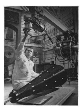
CARBON/CARBON nose cone, filamentwound, is x-rayed in the Nondestructive Testing Laboratory 7361 by Pete Peterson. The piece is checked for internal flaws before undergoing chemical vapor deposition in a furnace. Treatment at temperatures up to 2000°F may take as long as a week.
